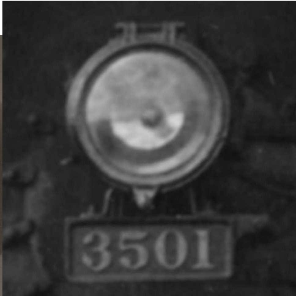
ESSCo Golden Glow Headlight Note top mounted hinge
